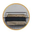
Added bracket on the panel cable connector to ensure it doesn't come loose8
